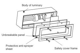
**Glazing:** special unbreakable material with anti-sprayer sheet
